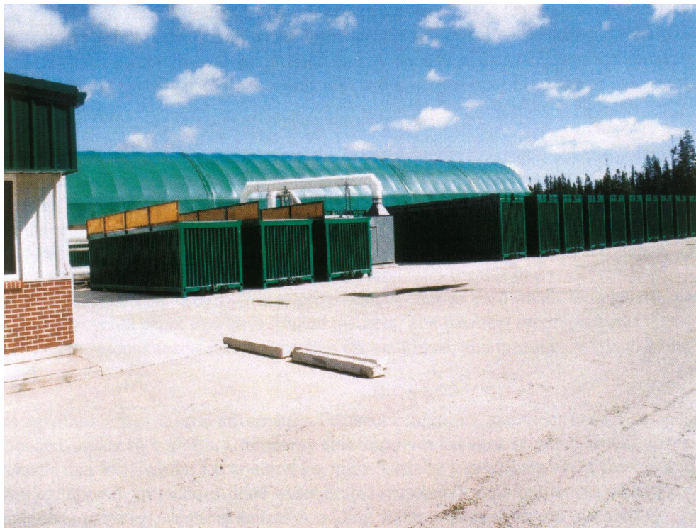
Photo 7-1: Typical In-Bin Composting System.
